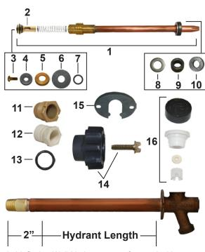
\*500 Series Wall Hydrants manufactured with a brass plated head (pictured above) and a nickel plated head.
